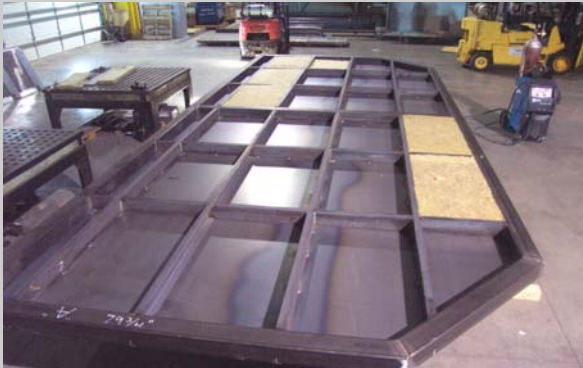
Custom Base Section Being Fabricated
