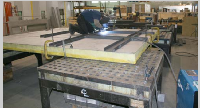
Custom Floor Section Being Fabricated
