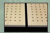
WoodTrends Custom for walls features a genuine wood plank treatment with perforations or grooves able to achieve NRC values as high as .90. The system is built on an MDF or chipboard core and the veneer is finished with 2 coats of a UV-polyacrylate lacquer. This system can be modified to suit your needs.
